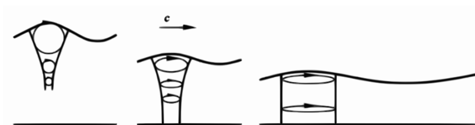
Fig. 4.6: Orbits of particle motion below a wavy water surface. Left: deep water; middle: intermediate water; right: shallow water.
